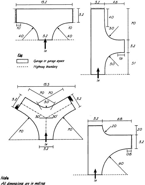
Dimensions shown are also the minimum requirements for car only turning within a cul-de-sac.
