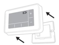
Remove old batteries and insert new ones.
