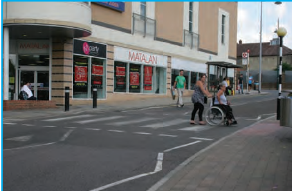
Zebra crossing on raised table.
