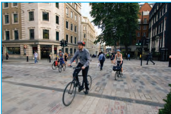
Signalised crossing on extensive raised table, City of London
